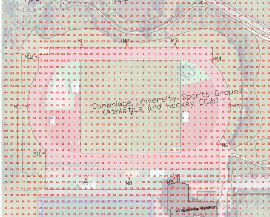
Figure 3: Existing Floodlighting Vertical Spill
